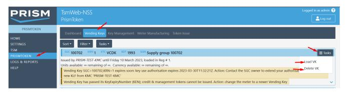
With vending firmware when the KEK Slot is in "Loading" state it is not possible to use the STS Vending commands. The key agreement session must be closed by selecting End Key Agreement Session which results in the KEK slot moving to the "Active" state which allows the STS Vending commands to be used.
